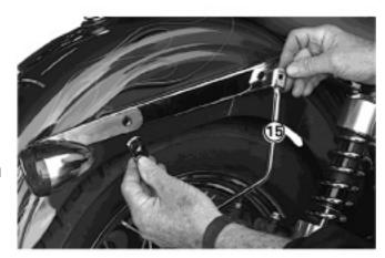
Attach the assembled bracket-turn signal assembly to the motorcycle using the supplied mounting bolt (16). After you have secured the bracket/turn signal assembly to the fender stay, tighten the turn signal mounting bolt (17) securely
